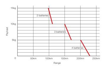
Range specified with 20% reserve energy in ideal conditions and no wind. Aircraft empty weight is 15 kg, maximum take-off weight is 40 kg Batteries are 5 kg each.
